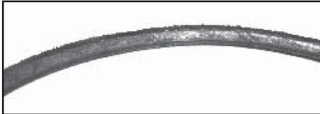
Shining surface due to high slippage
